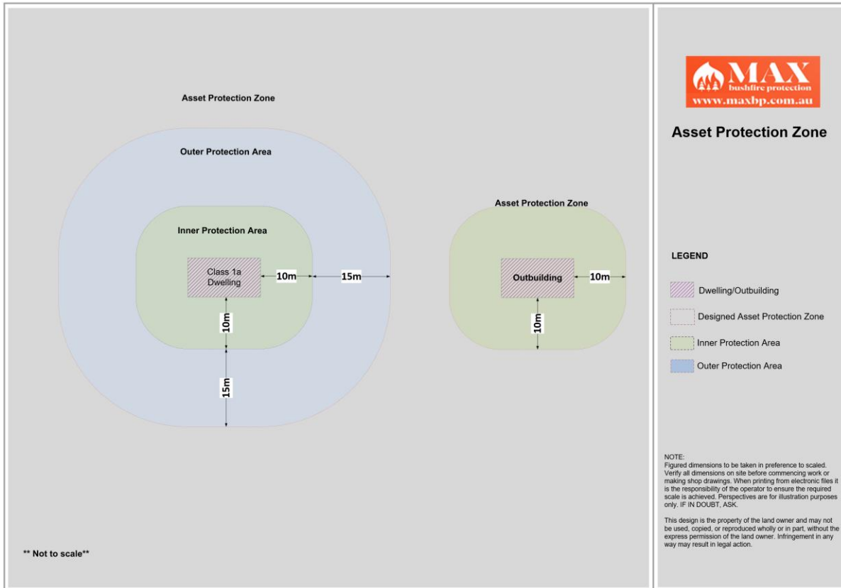
Figure 4-11: Asset Protect Zone – 25 m radius for new and existing Class 1a Dwelling
