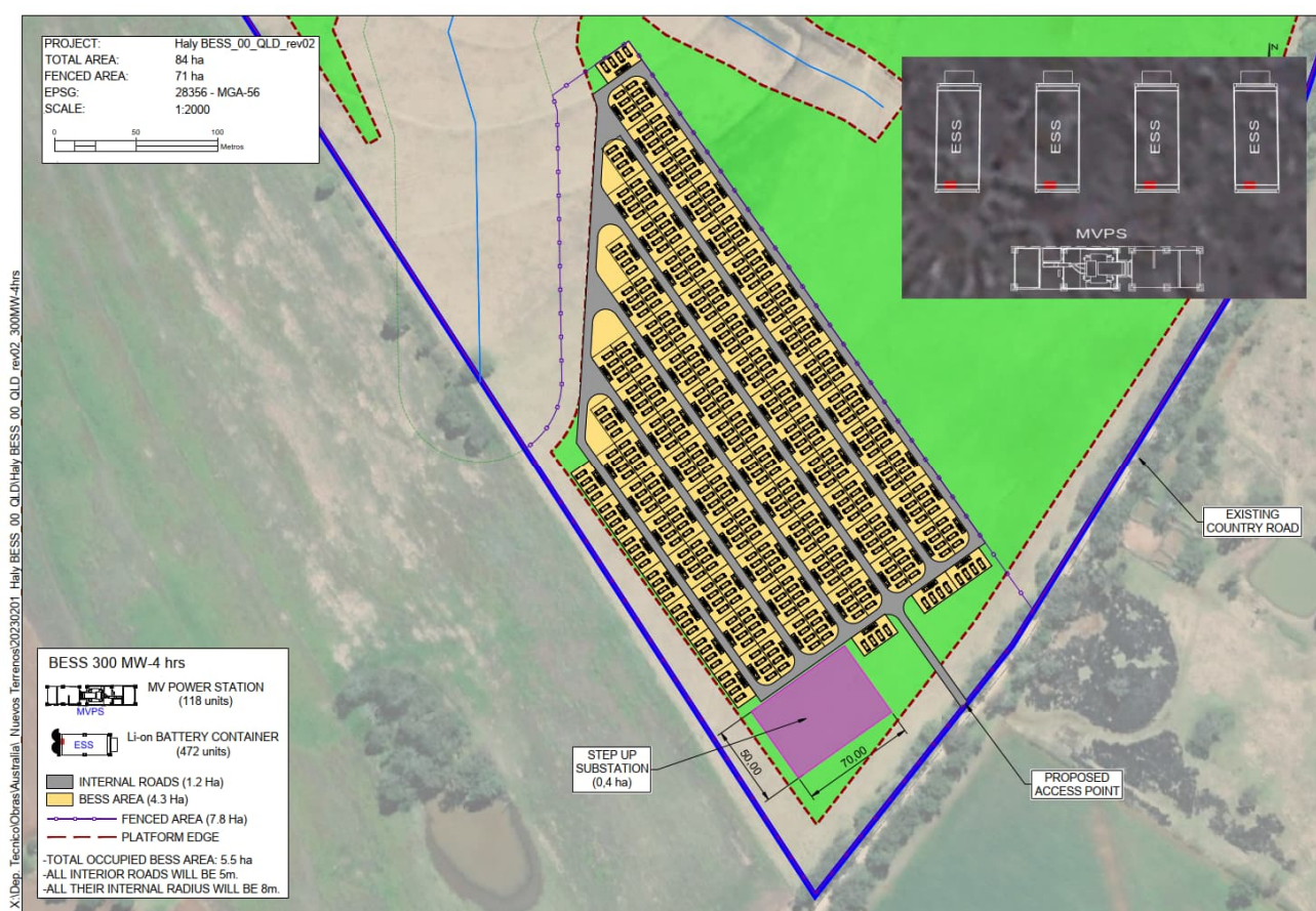
Figure 5.1 South Burnett BESS layout and Saft BESS block layout (indicative)
