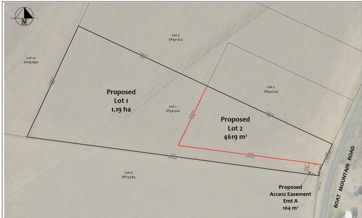
Figure 4: Plan of reconfiguration, Proposed Lots 1 and 2 and Easement A in Lot 1 on SP341224 (ONF Surveyors, Drawing No. 13968-P1).
