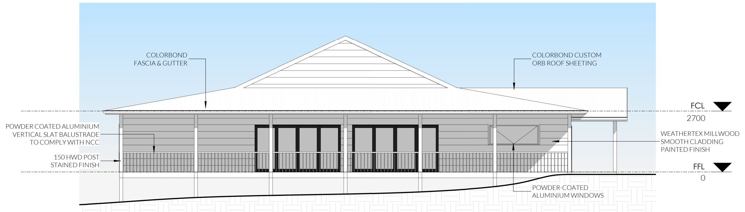
Elevation 2 - Function Building
