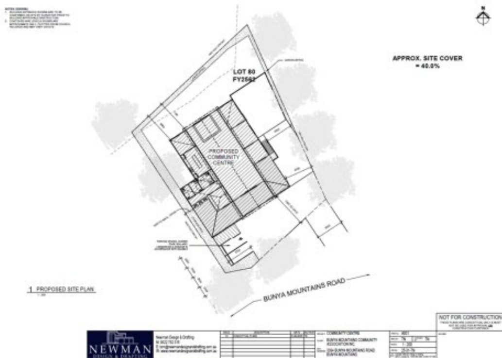
Figure 7 – Proposed Development Site Plan (Conceptual). (Source: Newman Design and Drafting, Drawn 05 June 2025).
