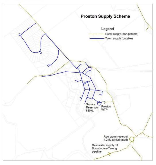
Council operates a non-potable rural supply scheme over an area 40 kilometres long in the Proston district. The non-potable scheme draws from the SunWater pipeline from Boondooma to Tarong. The raw water is chlorinated at a 1.2 ML hill-top reservoir south-east of Proston in order to control growths in the rural distribution pipework.
