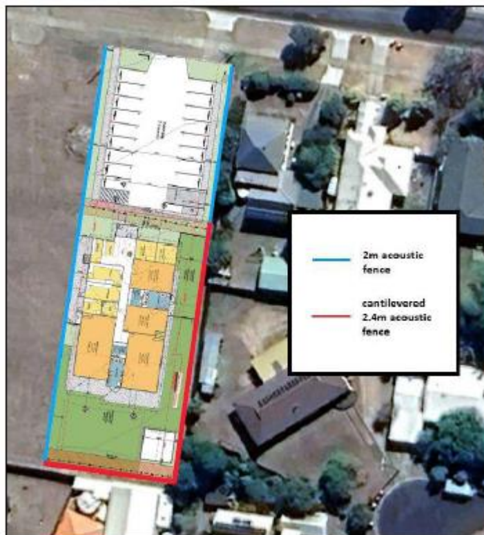
Amended Figure 1 – Recommended acoustic barrier specifications.
